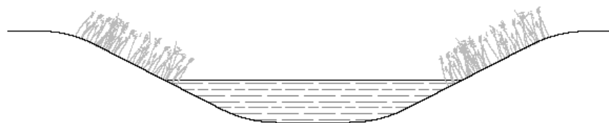
PROPOSED INDICATIVE GRADUAL SLOPING DITCH PROFILE
